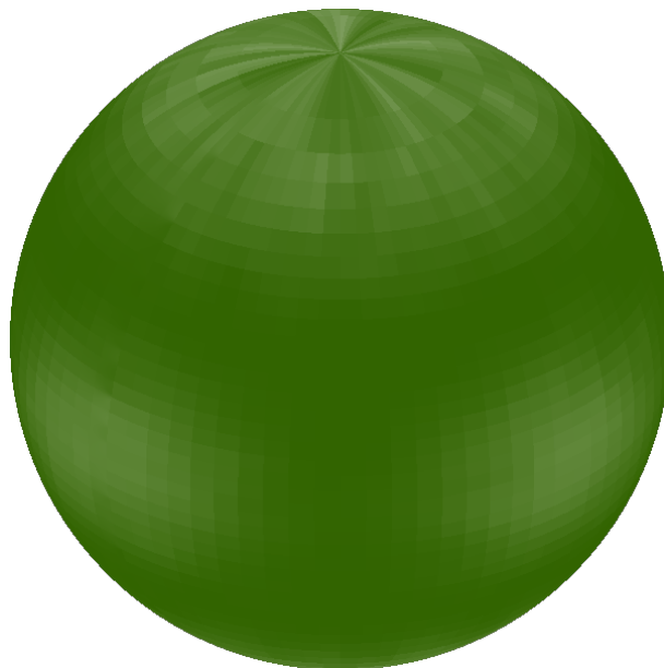
Figure 4.1: Example of a stereographic representation of the bond orientation function generated by RMCPProfile.
